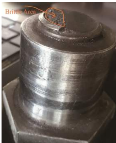
Fig.6 Brittle Area of the Fracture Surface
