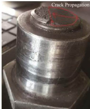
Fig.5 Process of Crack Propagation on the Fracture Surface
